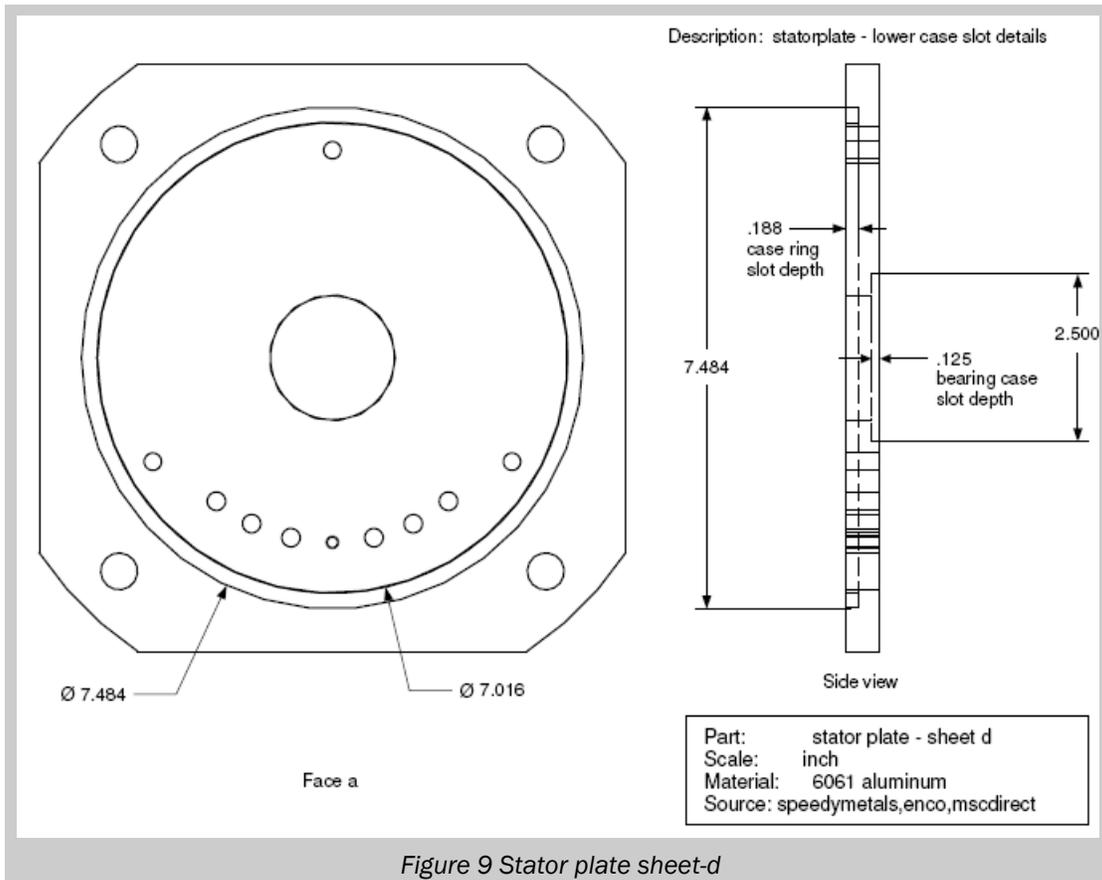
Figure 9 Stator plate sheet-d
