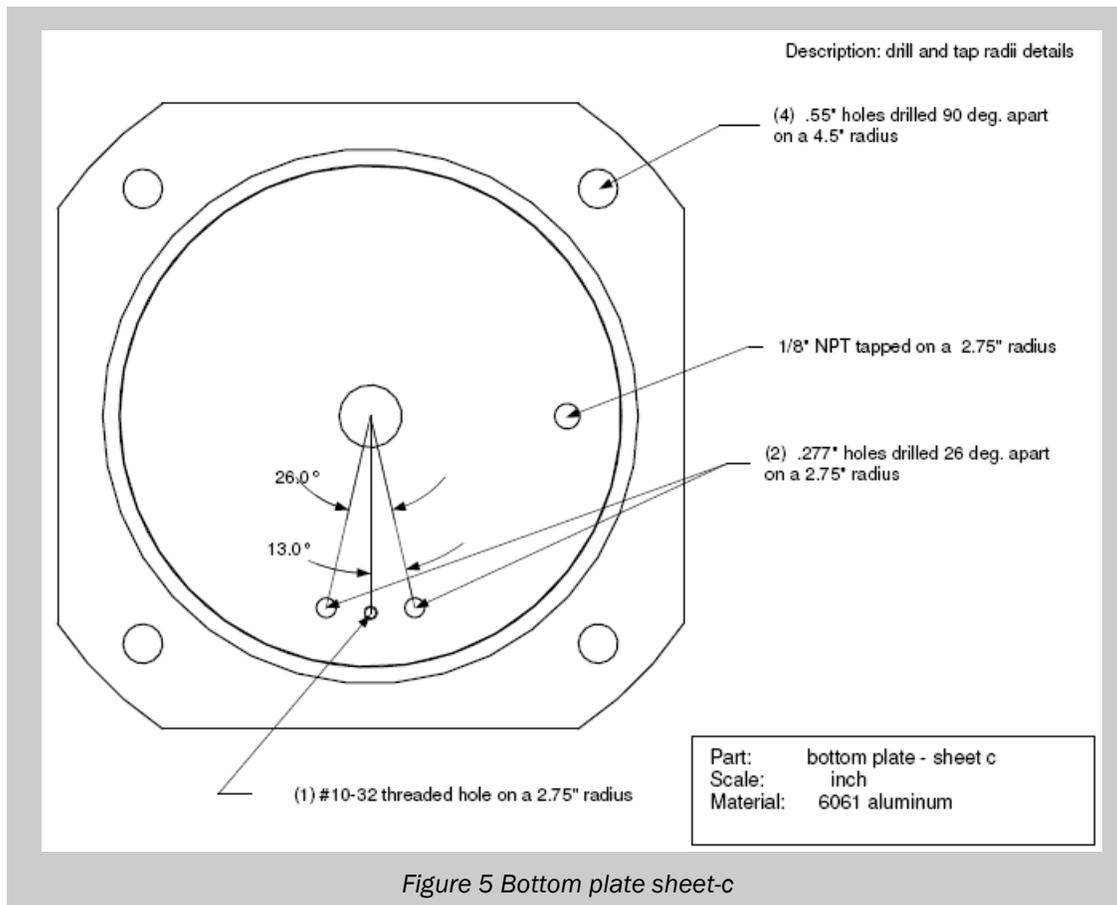
Figure 5 Bottom plate sheet-c
