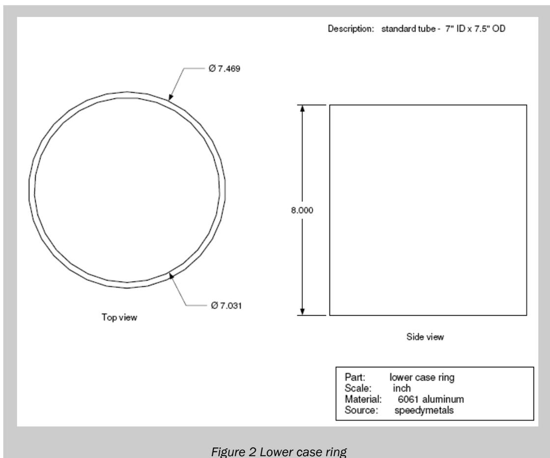
What I do to minimize the amount of material I have to remove is to first true up the tubing shape. Most tubing is manufactured out-of-round. I use a shop press (usually my mill) to compress the outer diameter that is the largest dimension, pushing down slightly past the 7.5" mark, letting it spring back to exactly 7.5" diameter.
