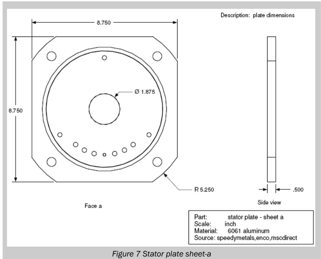
Figure 7 Stator plate sheet-a
