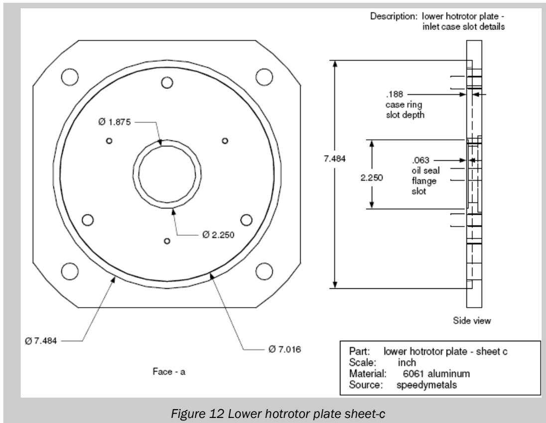
Figure 12 Lower hotrotor plate sheet-c
