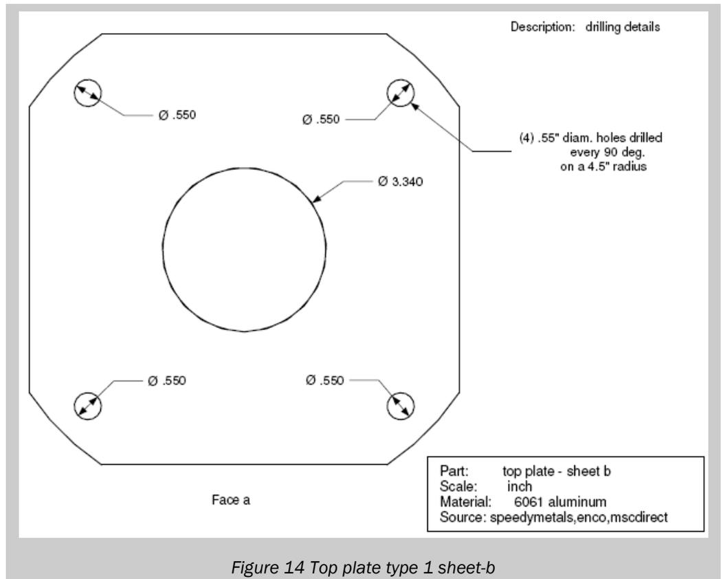
Figure 14 Top plate type 1 sheet-b
