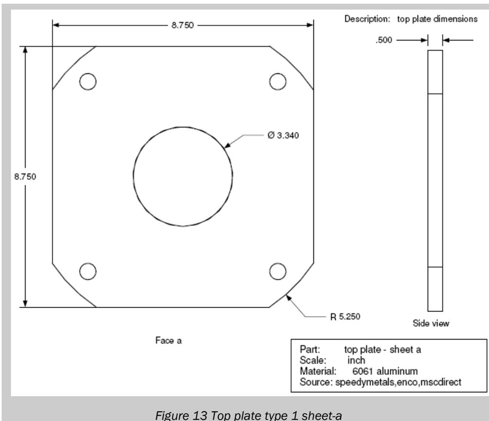
Figure 13 Top plate type 1 sheet-a
