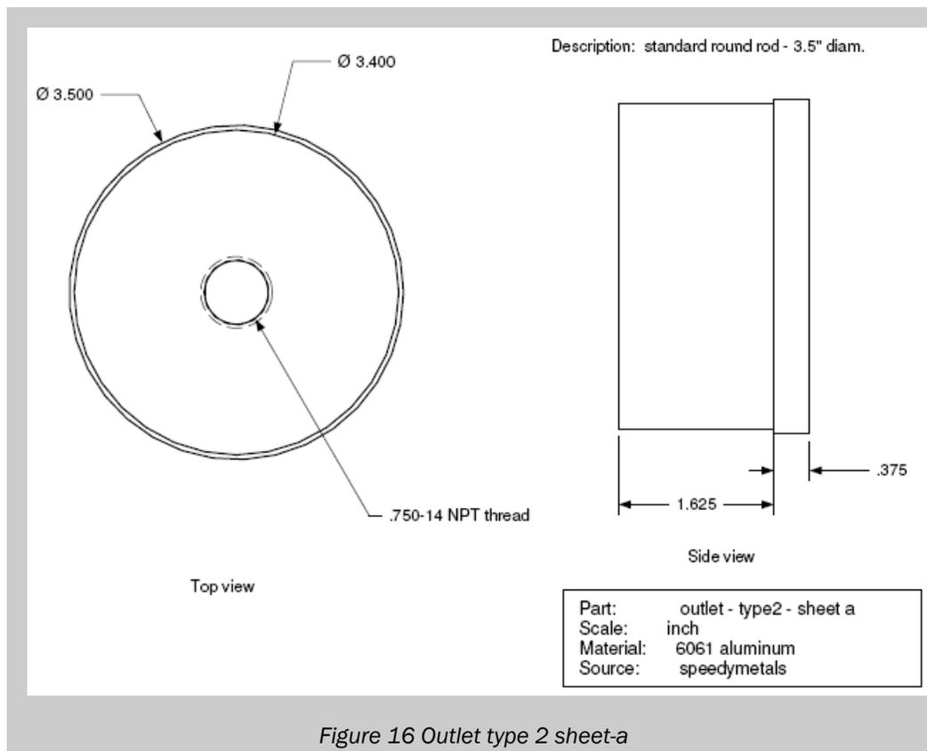
Remount the work piece in the chuck with the 3.5" O.D. end facing outward. Referring to the cross-section in *sheet-b*, first bore a 0.9375" hole through the rod.
