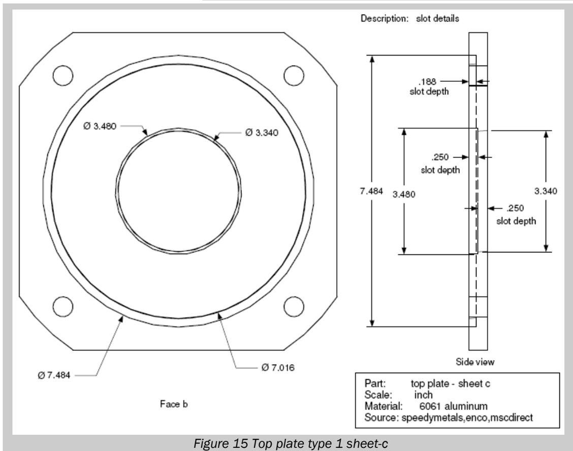
Figure 15 Top plate type 1 sheet-c
