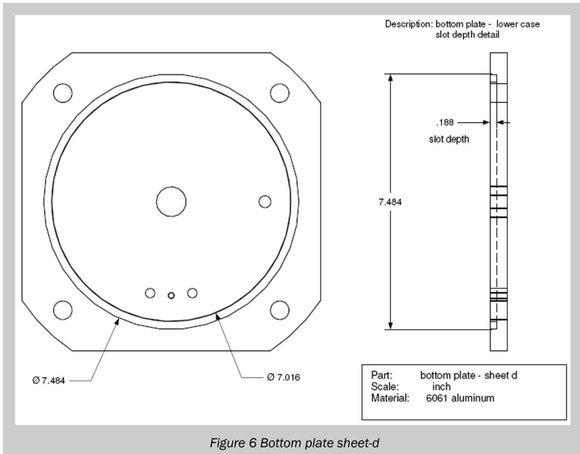
Figure 6 Bottom plate sheet-d
