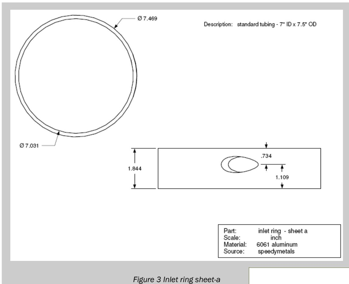
Figure 3 Inlet ring sheet-a
