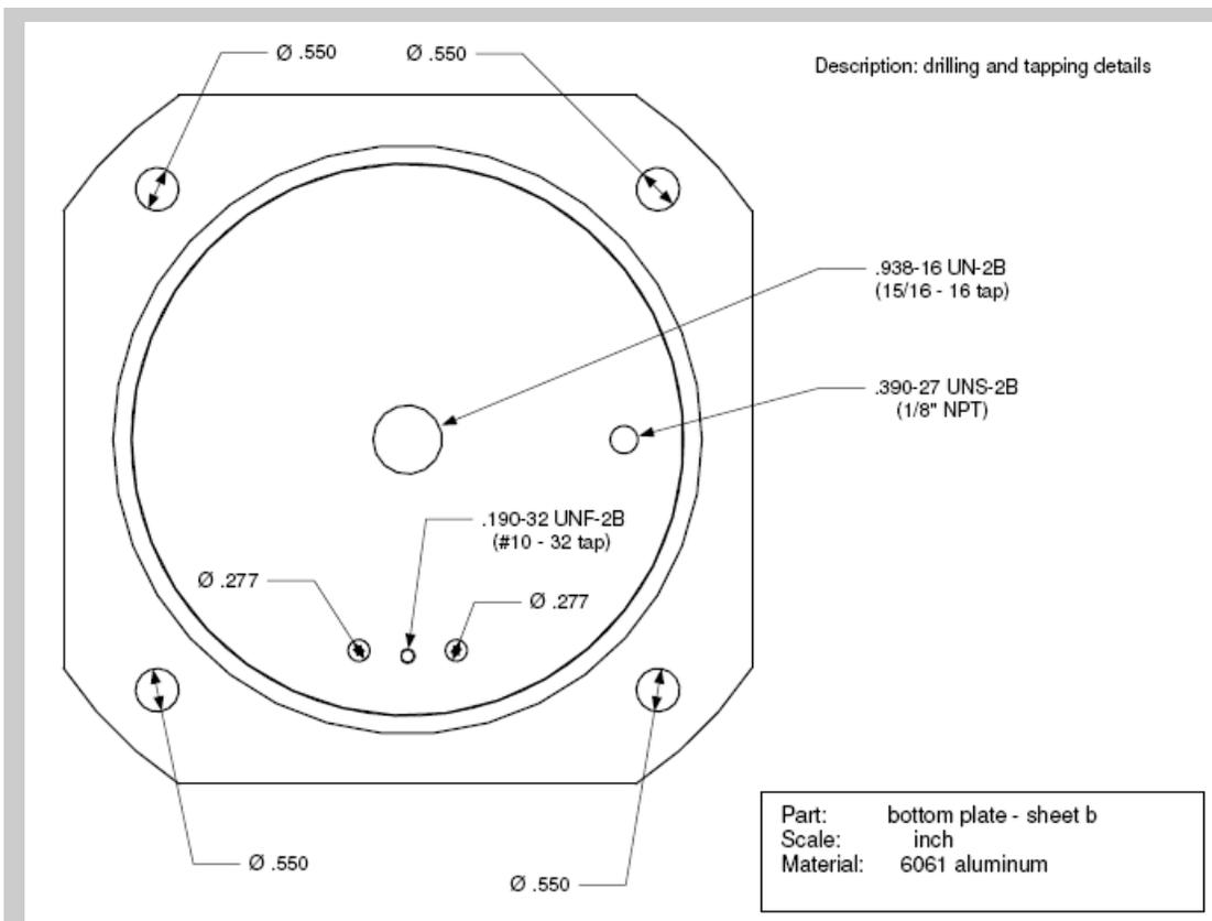
Mount one of the (4) plate blanks in an 8-inch 4-jaw chuck on the lathe. Most 4-jaw chucks have independent jaws so you can drift the work piece to align its center with the lathe tailpiece exactly.
