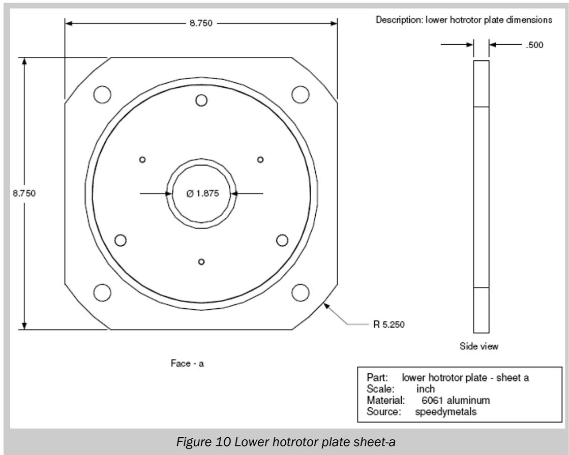
Figure 10 Lower hotrotor plate sheet-a
