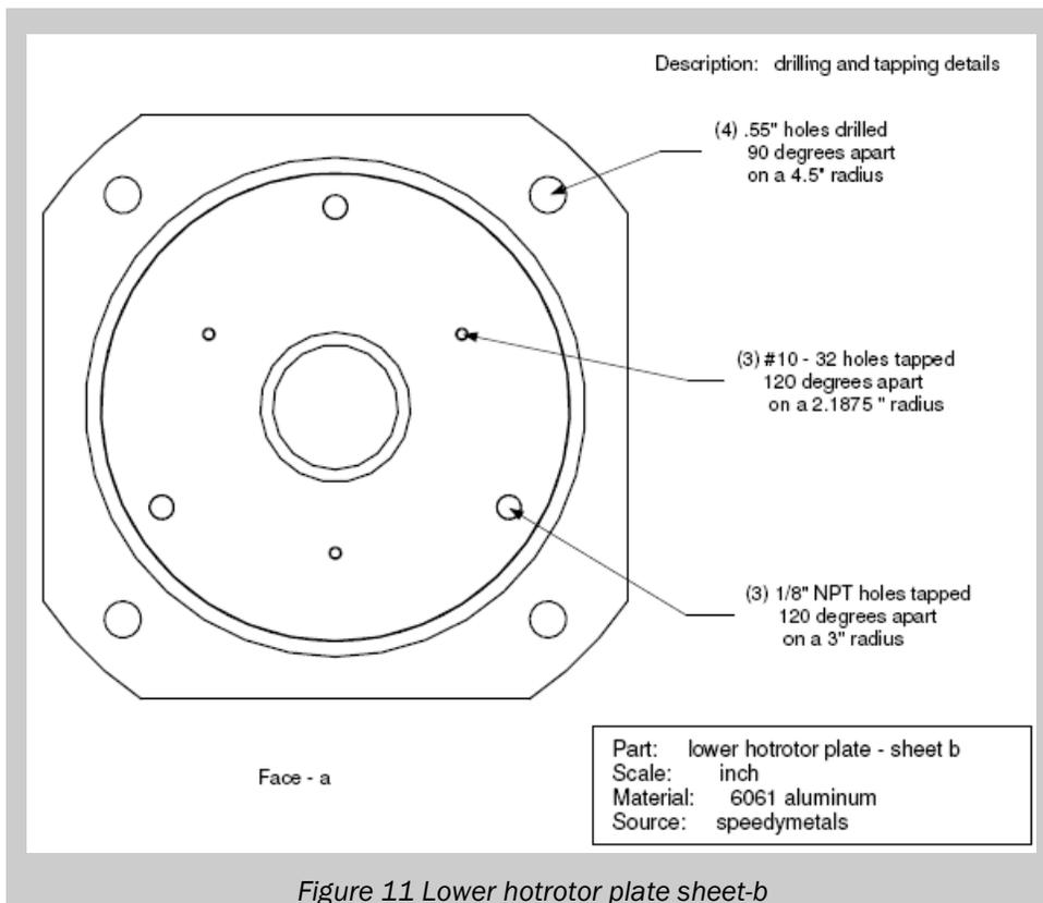
Figure 11 Lower hotrotor plate sheet-b
