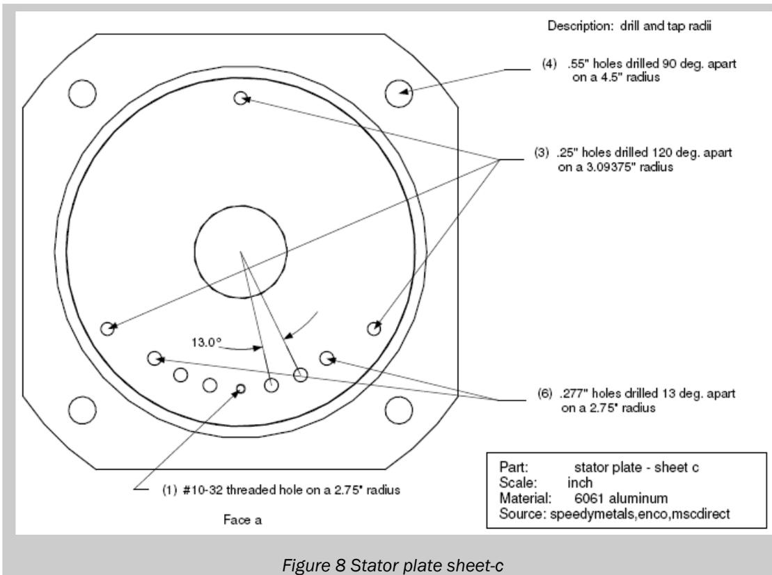
Figure 8 Stator plate sheet-c
