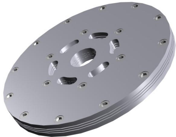
Figure 3 Hot rotor assembled
