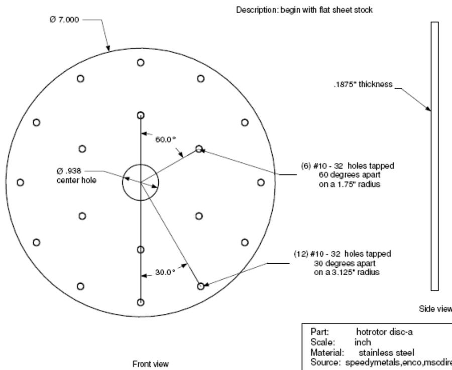
When I begin building a new hot rotor, I start with the bottom (back) plate (disc-a). The .125" holes are opened up with a #25 drill bit to .1495". A #10-24 or #10-32 tap is used (depending on the TPI threads of your #10 cap screws) to thread all 18 holes.
