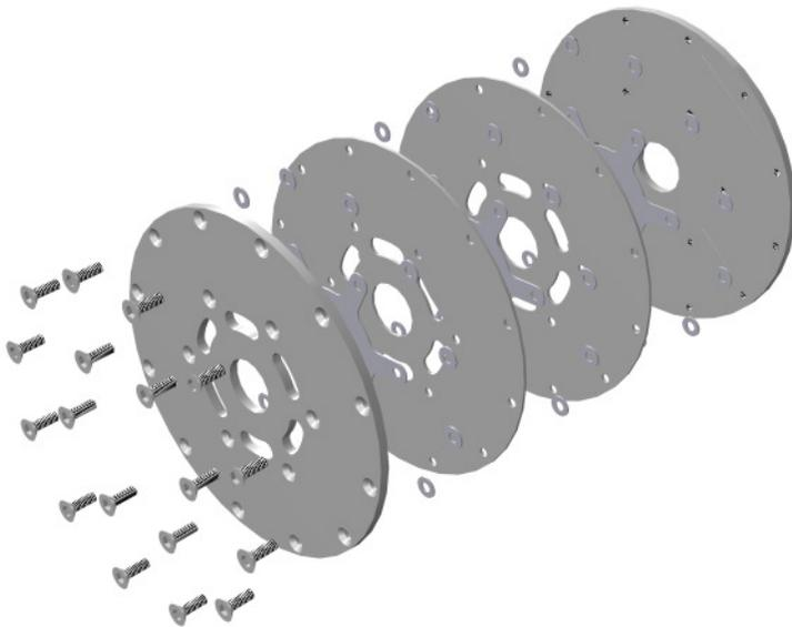
Figure 2 Hot rotor exploded view
