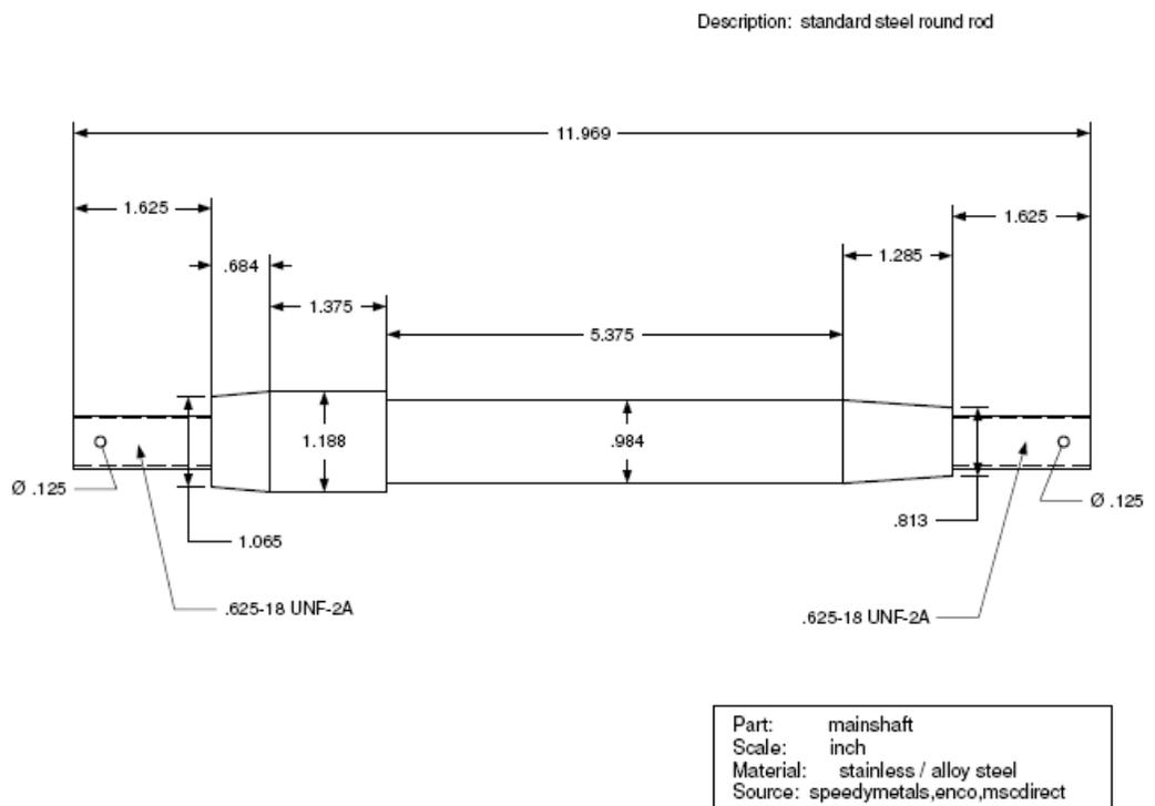
Figure 7 Main Shaft drawing
